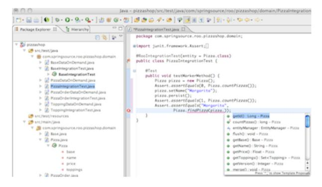
Note, most of the methods visible in the STS code assist are actually not in the Java sources but rather part of the AspectJ ITD and are therefore introduced into the Java bytecode at compile time.
