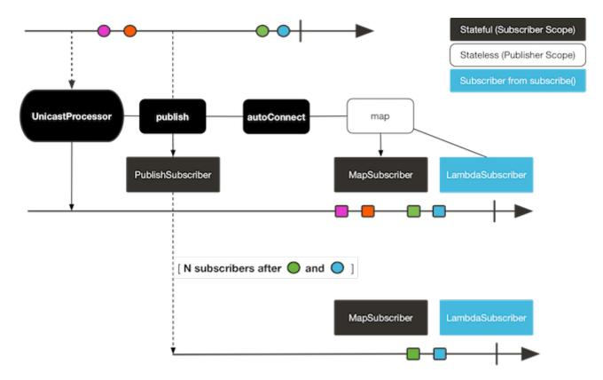
Subscriber 1 catches all four colors. Subscriber 2, having been created after the first two colors were produced, catches only the last two colors. This difference accounts for the doubling of ORANGE and PURPLE in the output. The process described by the operators on this Flux runs regardless of when subscriptions have been attached.
