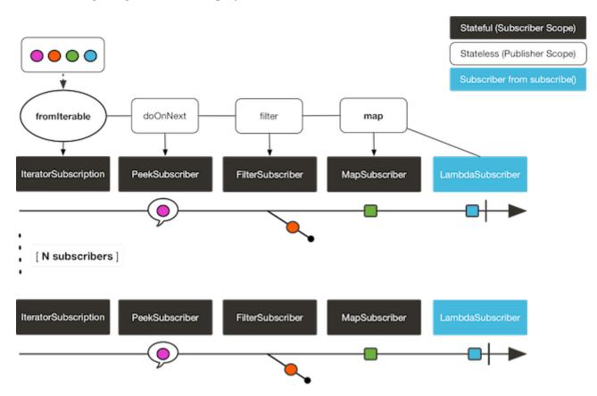
Both subscribers catch all four colors, because each subscriber causes the process defined by the operators on the Flux to run.
