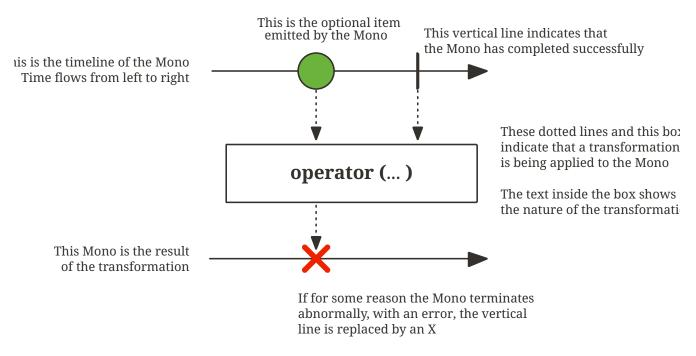
A Mono<T> is a specialized Publisher<T> that emits at most one item *via* the onNext signal then terminates with an onComplete signal (successful Mono, with or without value), or only emits a single onError signal (failed Mono).
