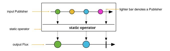
Note that sometimes we represent multiple variants or behaviors depending on the operator's input, in which case there's a single operator "box", but the source and output variants are separated like below:
