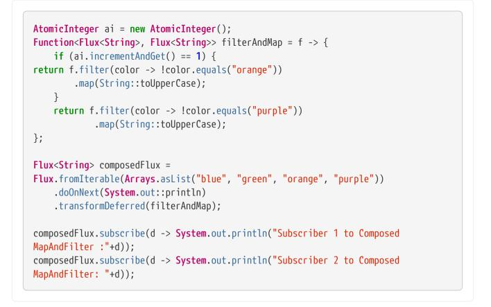
The following image shows how the transformDeferred operator works with per-subscriber transformations:
