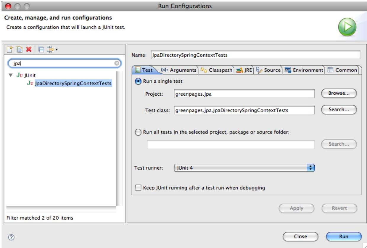
This test run will fail because there is no `DataSource` bean to be injected; it is typically sourced from the OSGi service registry at runtime:
