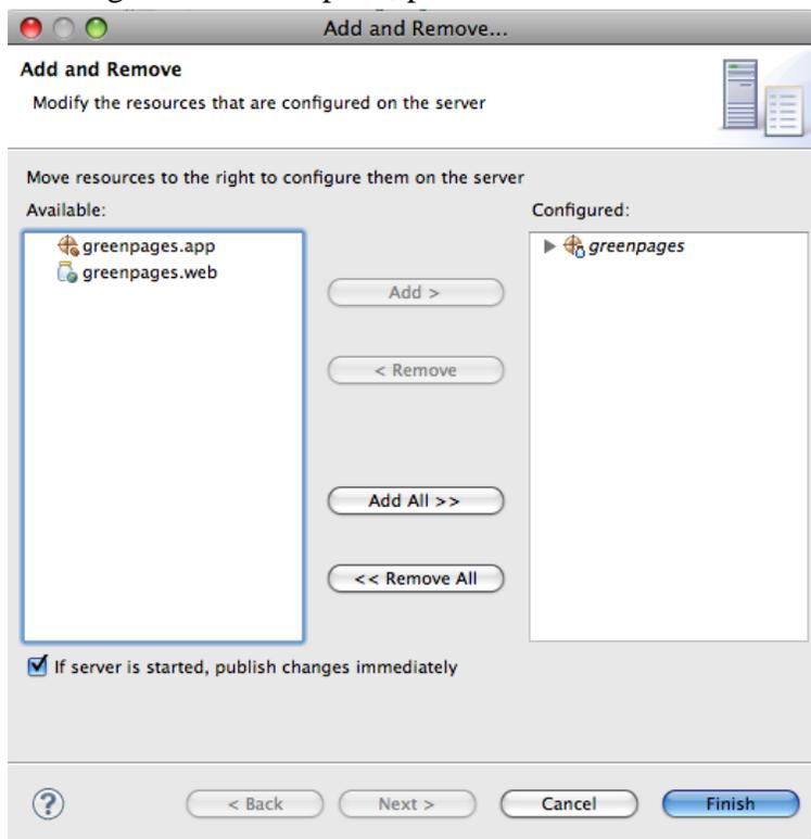
Eclipse automatically undeploys the `greenpages.web` bundle and deploys the `greenpages` PAR. When this happens, the deployment fails with an error. One of the exceptions in the exception list that is included is similar to:
