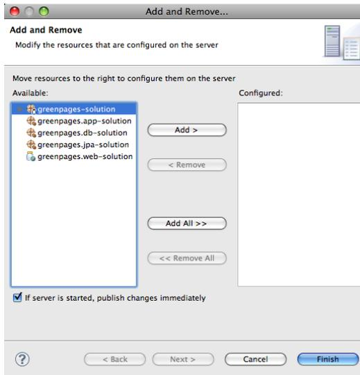
2. Add *greenpages-solution* (which is the containing project or PAR) to the server and finish.
