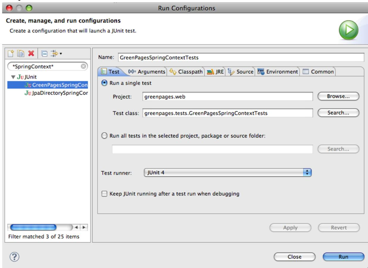
When this test is run, Spring creates an `ApplicationContext` that is built from the `module-context.xml` configuration files from all of the bundles. Because of this all of the internal dependencies are satisfied by the beans created directly by the bundles.
