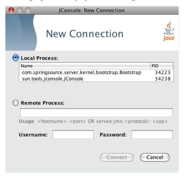
The following image shows how to specify a remote connection in JConsole that uses SSL with the default username/password (admin/springsource and default secure port of 9875).
