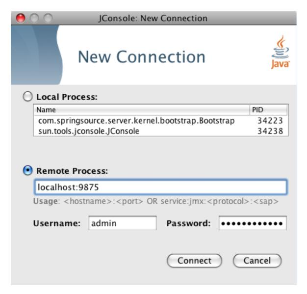
To start with the JMX remote access on a specific port number other than the default 9875, pass this port number in as the value of the -jmxport argument:
