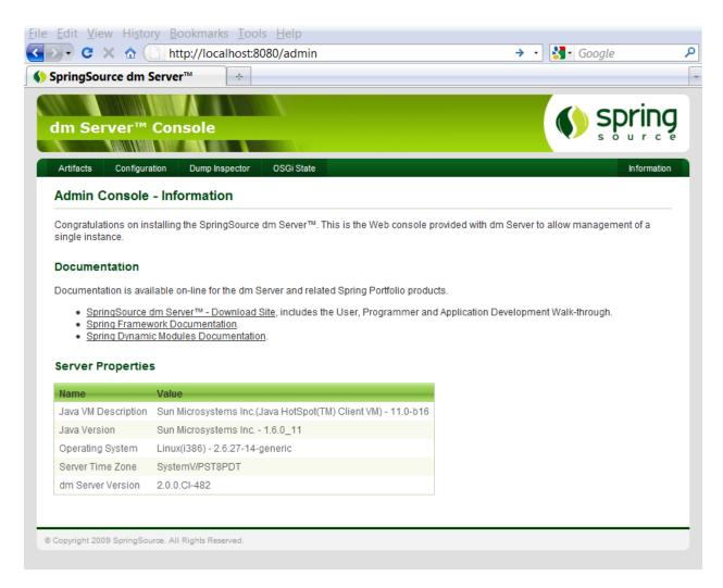
Use the links at the top of the console to perform various tasks, such as viewing and managing artifacts (**Artifacts**), viewing the properties of deployed configuration artifacts (**Configuration**), viewing details of dumps (**Dump Inspector**), and viewing the OSGi state of the dm Server instance (**OSGi State**).
