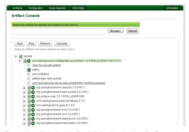
The particular details that the Admin Console displays depends on the artifact. For example, for all artifacts you can view their state and how it was installed (such as by a user using the Admin Console or programmatically). The two most common states are Active (running and ready to be used) and Resolved (all dependencies resolved but you must start it before you can use it.) An artifact can also be in one of the transition states, such as Starting and Stopping.
