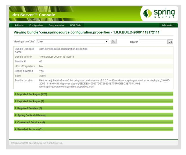
The console displays again the symbolic name, version, and internal ID of the bundle. It then displays whether the bundle is Spring powered and the exact physical location of the bundle JAR file on the computer that hosts dm Server.
