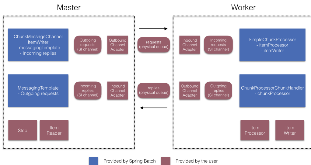
Figure 30. Remote Chunking Configuration
