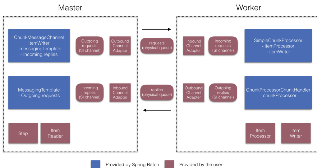
Figure 31. Remote Chunking Configuration
