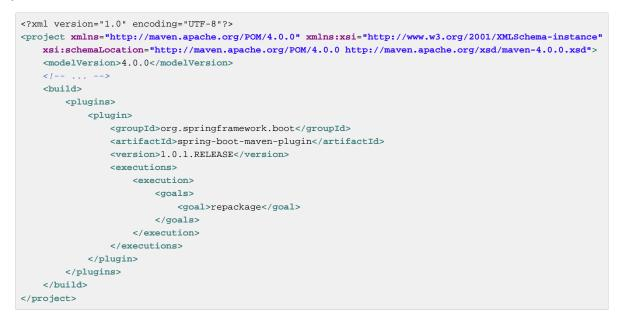
This configuration will repackage a jar or war that is built during the package phase of the Maven lifecycle. The following example shows both the repackaged jar, as well as the original jar, in the target directory:
