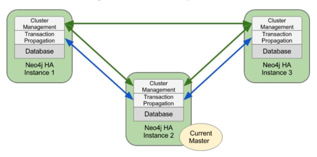
When operating in HA mode, Neo4j does not make open transactions available across all nodes in the cluster. This means we must bind every request within a specific transaction to the same node in the cluster, or the commit will fail with 404 Not Found.
