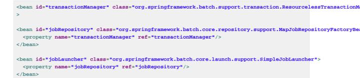
The declaration above define beans for JobRepository and JobLauncher. For simplisity we used in-memory repository while it would be possible to switch into repository working with a database if persistence is needed. A bean named jobLauncher is later used within the *Application Master* to launch jobs.
