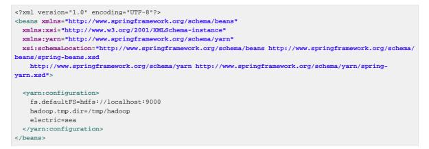
One can further customize the settings by avoiding the so called *hard-coded* values by externalizing them so they can be replaced at runtime, based on the existing environment without touching the configuration:
