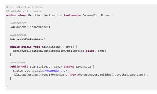
We used the @EnableBatchProcessing annotation to enable the batch features for Spring Boot.
