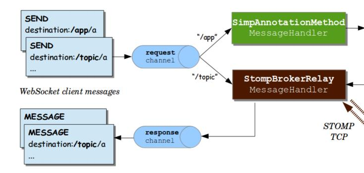
The main difference in the above diagram is the use of the "broker relay" for passing messages up to the external STOMP broker over TCP, and for passing messages down from the broker to subscribed clients.
