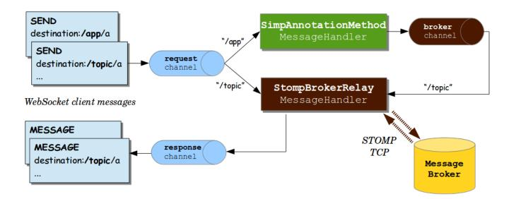
The main difference between the two preceding diagrams is the use of the "broker relay" for passing messages up to the external STOMP broker over TCP and for passing messages down from the broker to subscribed clients.
