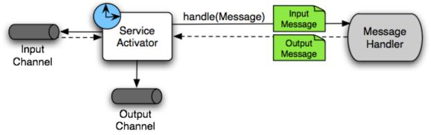
A request-reply "Service Activator" endpoint connects a target object's method to input and output Message Channels.
