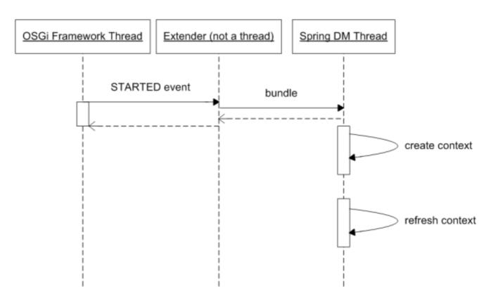
The extender considers only bundles successfully started, that is, bundles in *ACTIVE* state; bundles in other states are ignored. Therefore a Spring-powered bundle will have its application context created *after* it has been started. It is possible to force synchronous/serialized creation of application contexts for started bundles, on a bundle-by-bundle basis. See Section 6.1, "Bundle Format And Manifest Headers" for information on how to specify this behaviour.
