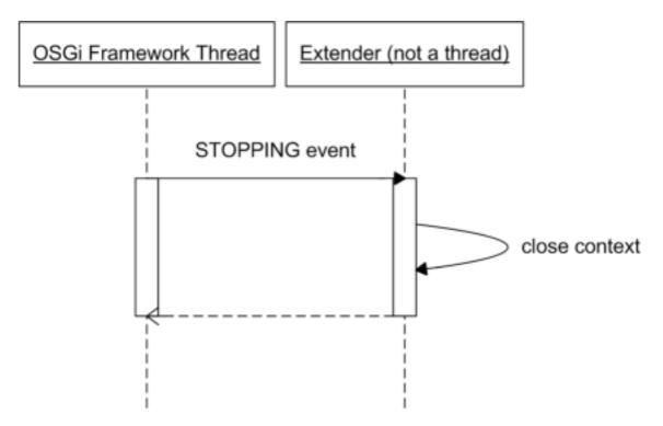
Note that a bundle can be closed individually or as part of a bigger event such as shutting down the entire OSGi platform. In this case or when the extender bundle is being closed down, the application contexts will be closed in a managed manner, based on the service dependencies between them. Please see the next section for more details.
