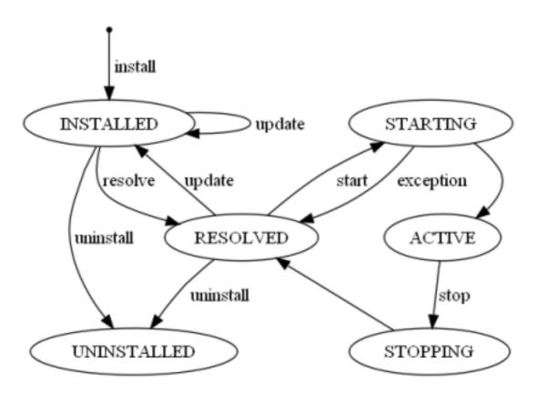
The OSGi PackageAdmin refreshPackages operation refreshes packages across the whole OSGi framework or a given subset of installed bundles. During the refresh, an application context in an affected bundle will be stopped and restarted. After a refreshPackages operation, packages exported by older versions of updated bundles, or packages exported by uninstalled bundles, are no longer available. Consult the OSGi specifications for full details.
