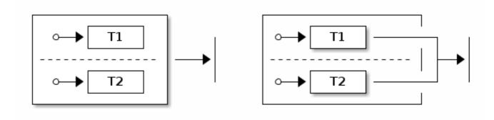
Source state can be a parent state hosting regions, which means that join states will be a terminate states of a participating regions. It's also possible to define source states to be any state in a regions which allows controlled exit from a regions.
