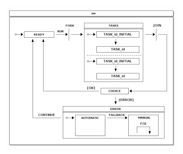
Executing a Runnable may result an error and especially if a complex DAG of tasks is involved it is desirable that there is a way to handle tasks execution errors and then having a way to continue execution without executing already successfully executed tasks. Addition to this it would be nice if some execution errors can be handled automatically and as a last fallback, if error can't be handled automatically, state machine is put into a state where user can handle errors manually.
