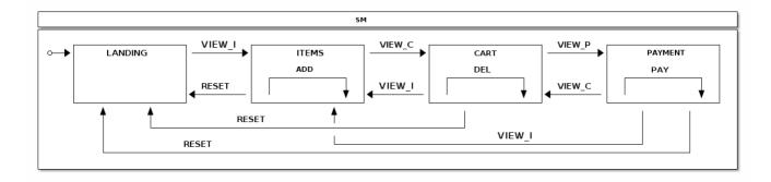
In below state machine configuration we simply model what we have in a state chart. Various actions are updating state machine Extended State to track number of entry's into various states and also how many times internal transition for ADD and DEL are called and if PAY has been executed. Don't focus on stateMachineTarget or @Scope for now, as we'll explain those in a bit.
