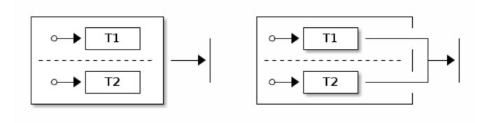
Source state can be a parent state hosting regions, which means that join states will be a terminate states of a participating regions. It's also possible to define source states to be any state in a regions which allows controlled exit from a regions.
