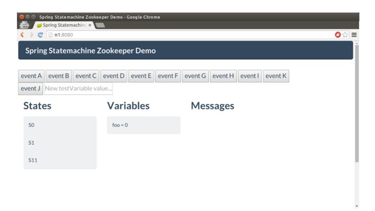
When you press button  $Event\ C$  in any of a browser window, distributed state is changed to S211 which is the target state denoted by transition associated with an event C.
