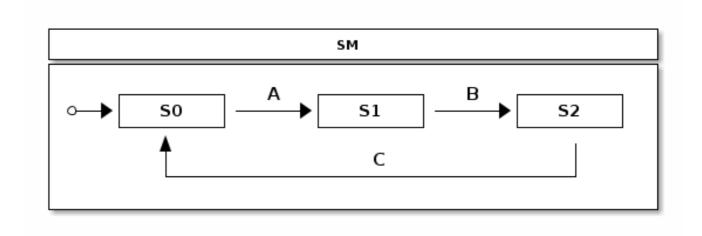
This is a simple state machine having states S0, S1 and S2. Transitions between those are controlled via events A, B and C as shown in a state chart.
