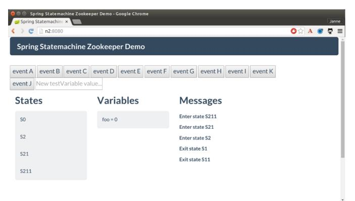
Then let's press button Event H and what is supposed to happen is that internal transition is executed on all state machines changing extended state variable foo from value 0 to 1. This change is first done on a state machine receiving the event and then propagated to other state machines. You should only see variable foo to change from 0 to 1.
