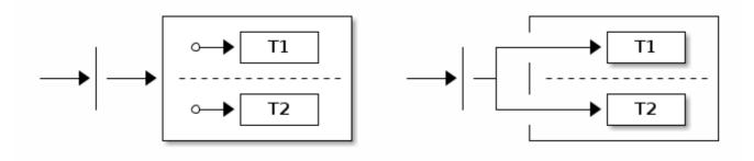
Target state can be a parent state hosting regions, which simply means that regions are activated by entering its initial states. It's also possible to add targets directly to any state in a region which allows more controlled entry into a state.
