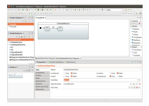
From state you want to link(in this case state S2), click Submachine field and choose your linked machine, i.e. SubStateMachine.
