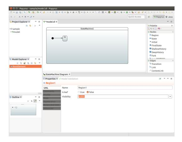
In above we added one state S1, initial state, and draw a transition between those two to indicate that S1 is an initial state.
