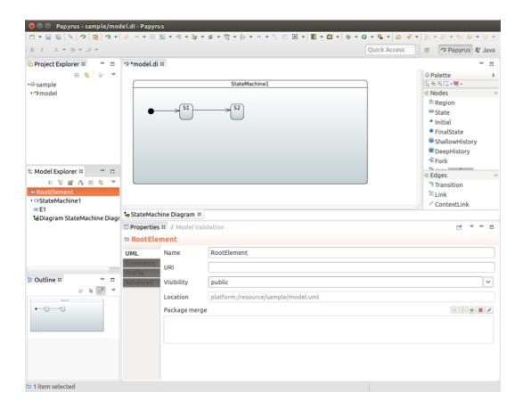
And then SignalEvent with defined signal E1. Done from RootElement#New Child#SignalEvent.
