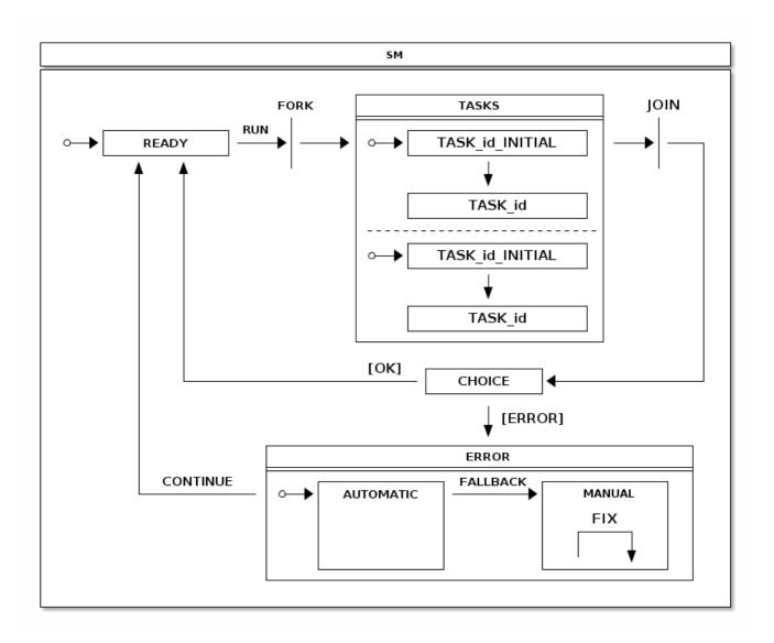
Executing a Runnable may result an error and especially if a complex DAG of tasks is involved it is desirable that there is a way to handle tasks execution errors and then having a way to continue execution without executing already successfully executed tasks. Addition to this it would be nice if some execution errors can be handled automatically and as a last fallback, if error can't be handled automatically, state machine is put into a state where user can handle errors manually.
