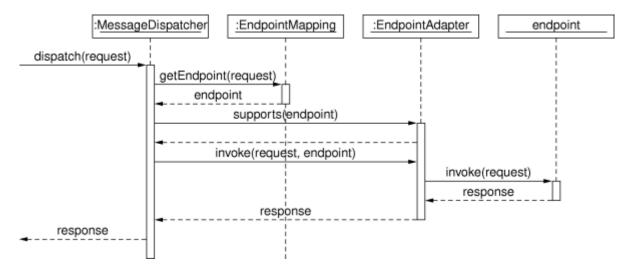
When a MessageDispatcher is set up for use and a request comes in for that specific dispatcher, the MessageDispatcher starts processing the request. The following process describes how
