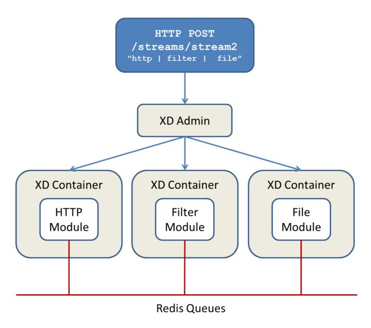
Figure 7.9. Distributed HTTP to Filter to File Stream
